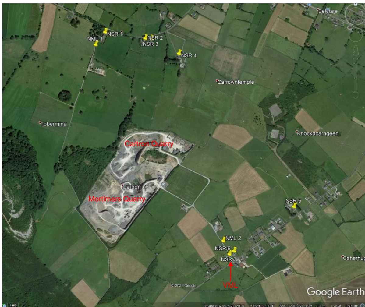
Figure 8.1: Noise Monitoring Locations (NML 1 & 2), Vibration Monitoring Location (VML) and Noise Sensitive Receiver (NSR 1- 7) locations included in the noise prediction model.
